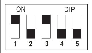
Dip switches 1 to 4 are for channel selection. Switch 5 lets you set up the auto-sequence timer for four cameras on four different channels to monitor a series of rooms for maximum supervision of the house (or office).  $\mathcal{Y}$
